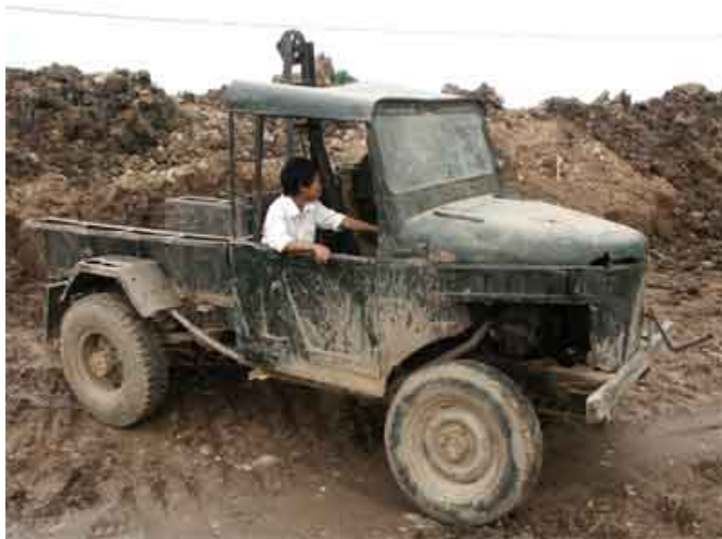
A "UN" truck, so named by locals because it was manufactured from spares from all trucks at a scrap yard. Note engine starting crank.
